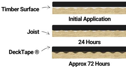
DeckTape® becomes gradually stronger over 24-72 hours as the adhesive soaks into the timber and fully cures.
