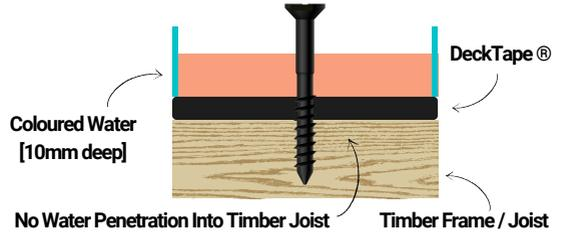
Completely self-sealed when fastener is driven through the DeckTape®
